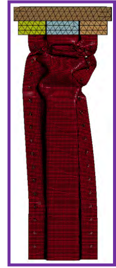
Progressive Folding: 1 SW failure (Damage + Reg. + SW Failure)
