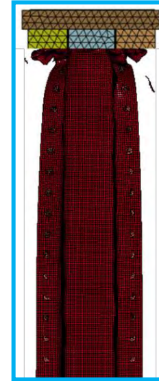
Progressive Folding (Damage without Reg.)
