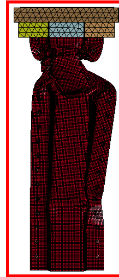
Mixed Buckling/ Folding (No Damage Model)
