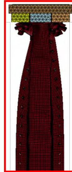
Progressive Folding (No Damage Model)
