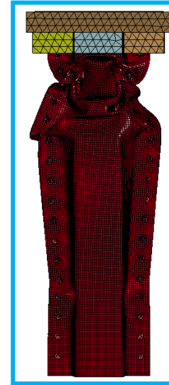
Mixed Buckling/Folding (Damage without Reg.)
