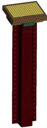
Axial Crush Model (full symmetry)
