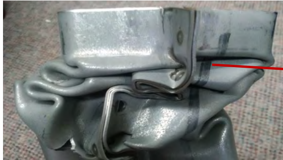
DP980 Material 2 Global Buckling and Folding
