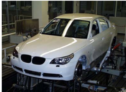
Body in White incl. Wind Screen, Doors, Hoods, Bonnet, axle carrier, crash beam, and other parts which are relevant for durability behavior
