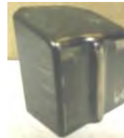
M4 Insert Coated w/ TiC
