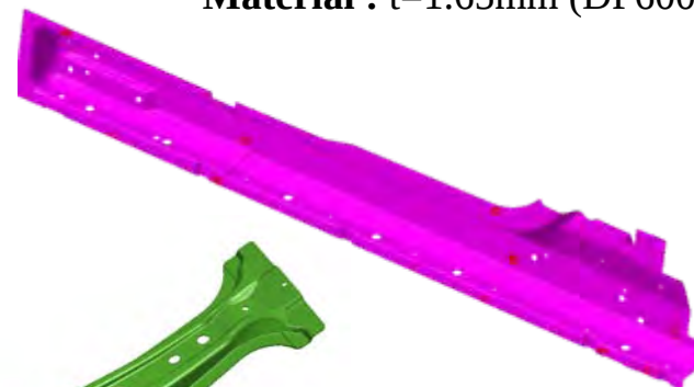
ROCKER REINF. (year 2003) Material : t=1.65mm (DP600)
