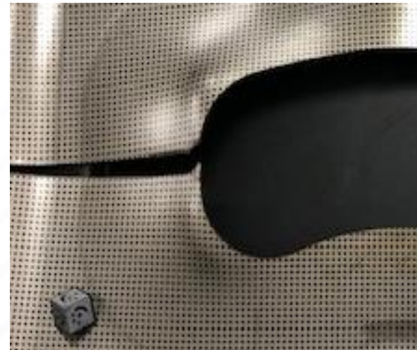
GEN3-980 sample punched with 12% clearance
