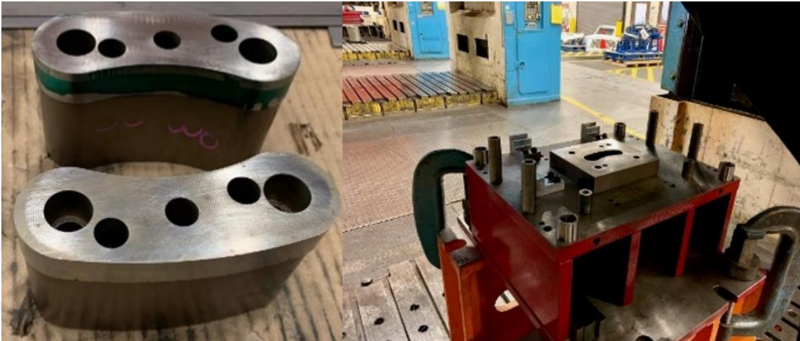
Peanut-shaped punches (left) and punching test tooling (right)
