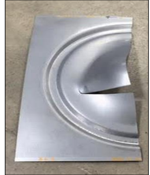
1.4-mm TRIP780 with the Sheared Edge
