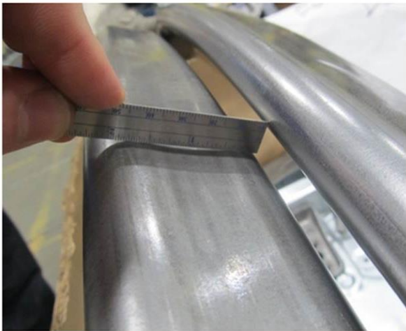
Too much compensation (Concave part surface)
