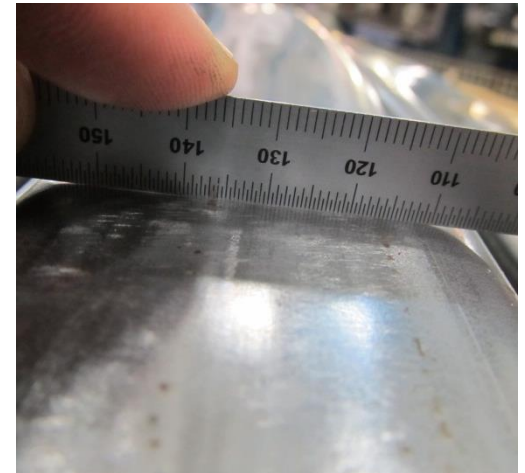
Correct compensation (Straight surface)
