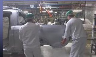
Rr Fender Install
