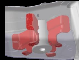
Collar + butterfly braces (+45% mount stiffness)
